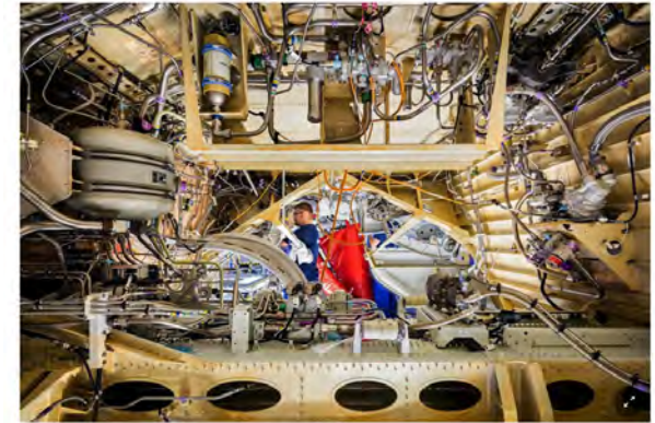
A look inside a main landing-gear wheel well. At this station, the aircraft is fitted with the vertical and horizontal stabilizers and the tail cone. This is also where the landing-gear doors, the radar and the navigation antennas are installed. (Illustration: Peter for The New York Times)
