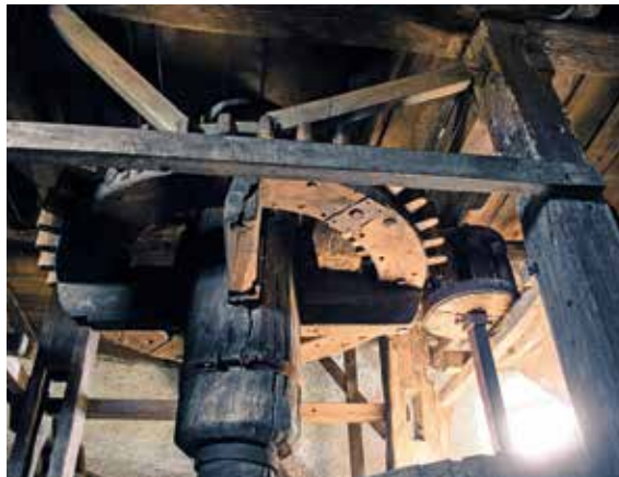
Wooden gears transferred power from the blades to the grinder in windmills.
